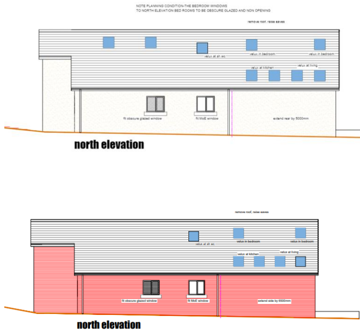
Figure 5: Existing v proposed north elevation details
